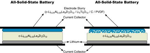
Figure 1. Schematic drawing of a) nonmodified all-solid-state battery and b) interface-engineered all-solid-state battery based on c-Li<sub>6.25</sub>Al<sub>0.25</sub>La<sub>3</sub>Zr<sub>2</sub>O<sub>12</sub> solid electrolyte, and Li<sub>4</sub>Ti<sub>5</sub>O<sub>12</sub> and Li-metal electrodes.
