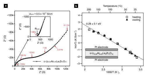
Figure 3. a) Nyquist plot of a c-Li<sub>6.25</sub>Al<sub>0.25</sub>La<sub>3</sub>Zr<sub>2</sub>O<sub>12</sub> pellet with Pt electrodes measured at room temperature. b) Arrhenius plot for heating and cooling cycles of the bulk ionic conductivity of c-Li<sub>6.25</sub>Al<sub>0.25</sub>La<sub>3</sub>Zr<sub>2</sub>O<sub>12</sub>. (Inset) Measurement schematic displaying c-Li<sub>6.25</sub>Al<sub>0.25</sub>La<sub>3</sub>Zr<sub>2</sub>O<sub>12</sub> pellet with symmetric platinum electrodes.
